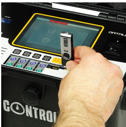
Data acquisition unit DATALOG 8 model 82-P9008/F - Detail of the 6.5" touch screen colour graphic display
