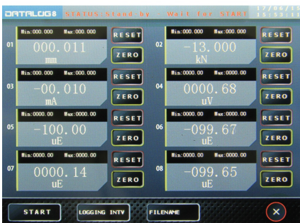
Data acquisition unit DATALOG 8 model 82-P9008/F - Live readings of the 8 channels
